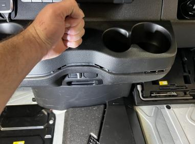
You can reinstall the cup holders at this time. Place the cup holders back into position, and give it a solid tap to seat it into place.
