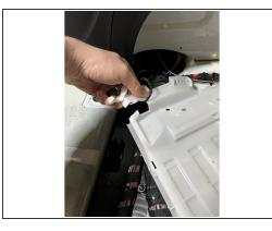
To finish remove the wire chase cover, it is necessary to loosen the drivers side seat base to allow the chase to be completely removed.
