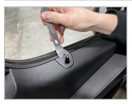
Remove the lock actuator rod cover by using a trim removal tool to work it free.
