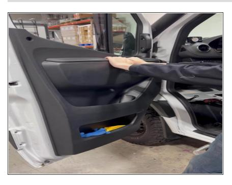
With all the fastners removed, you can now remove the door panel. The best way is to firmly grasp the door grab handle, and give the panel a rapid and hard pull. The door panel will pop free.
