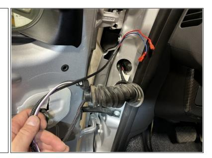
Feed the harness through the pass thru grommet. This can be a tad challenging, it is easiest to compress the grommet, and use one hand to feed the wires, and the other to try to fish the wires out of the other-side of the grommet.
