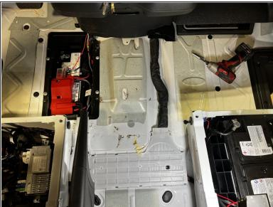
Remove the two nuts securing the wire chase cover that runs forward to rear using a 10mm socket and wrench. Set the cover and nuts aside.
