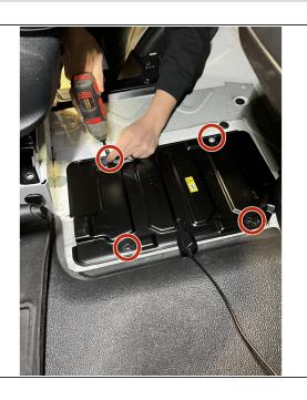
Locate the 4 screws that secure the battery tray cover. Use a T30 Torx bit to remove the screws. Lift up on the cover to remove.
