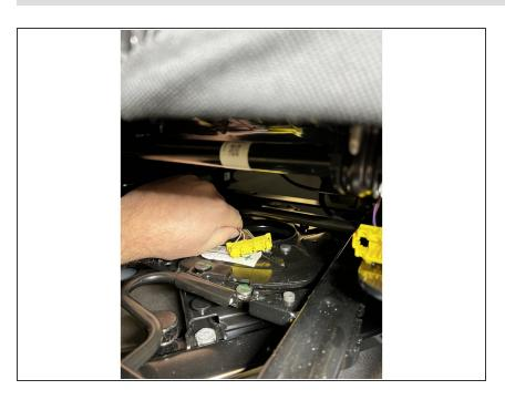
Route seat wire harness and the power seat harness (if equipped) through the opening in the seat swivel.
