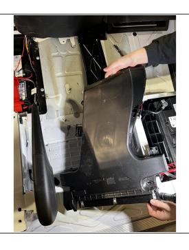
With the fasteners removed, lift up on the forward section, and gently work it free from the connection point under the dash board. Once the forward section is removed, you can remove the rear section. Set both sections aside.
